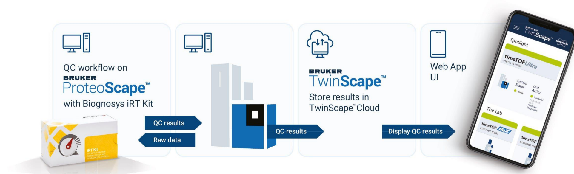
Fig. 1. Overview of the quality management workflow integrating Biognosys iRT kit, Bruker ProteoScape data processing and automated upload and monitoring with TwinScape.
