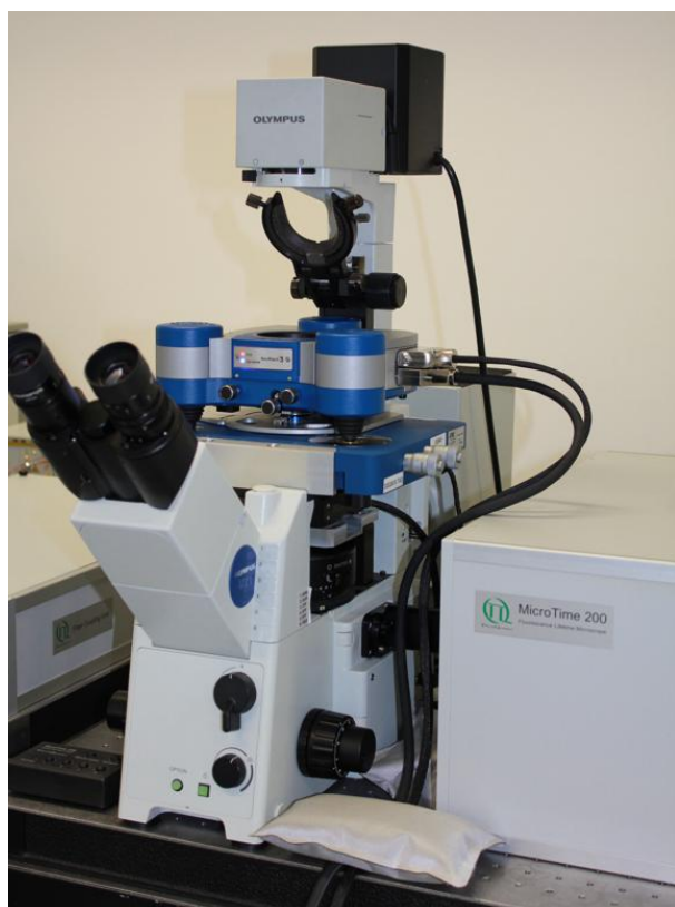
Fig. 1: Combined setup of MicroTime 200 and JPK NanoWizard ® 3 AFM. The AFM sample stage (TAO ™ module, 3-axis) is mounted to the IX71 body of the MicroTime 200. The MicroTime 200 is configured for 2D objective scanning.
