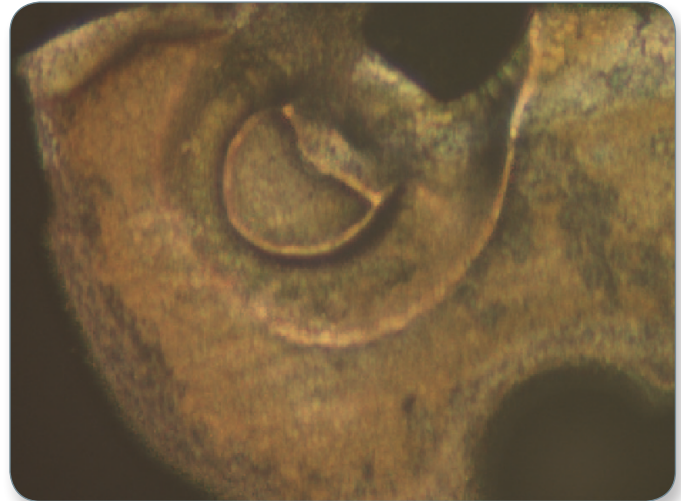
Figure 10. WLI microscopes can now produce color images, as seen here for wire bonding characterization.
