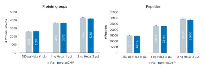
**Repetitive injections of different peptide concentration** (250 pg, 1 ng or 2 ng) of a HeLa cell lysate digest either injected from an autosampler vial (grey) or from the proteoCHIP (blue) (25 min total run time) with indicated volumes pipetted into each well show excellent reproducibility on protein group (A) and peptide (B) level.
