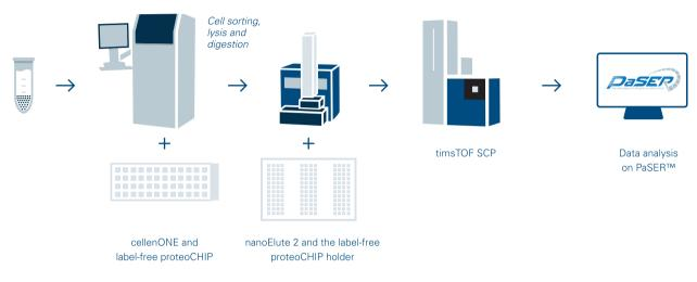
Fully automated label-free single cell proteomics workflow using the cellenONE with the lable-free proteoCHIP and with holder support in the nanoElute 2 for ultra-sensitive single cell analysis on the timsTOF SCP and data analysis on the PaSER™ using TIMS-DIA-NN.
