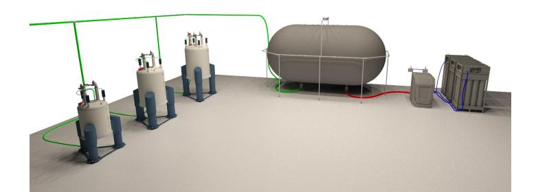
This solution with a big balloon is ideal for customers who have the ability to liquefy helium, either in their own labs or with the help of external collaborators. It can collect the boiloff of many NMR magnets in parallel, including helium transfer losses.
