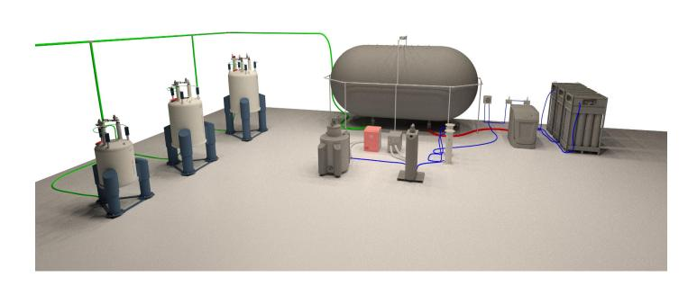
This solution with a big ballon plus a purifier and liquefier allows for a full high-pressure recycling loop. The collected helium gas is reliquefied and can be reused, making it an ideal solution for customers who want to be as independent from liquid helium supply as possible.
