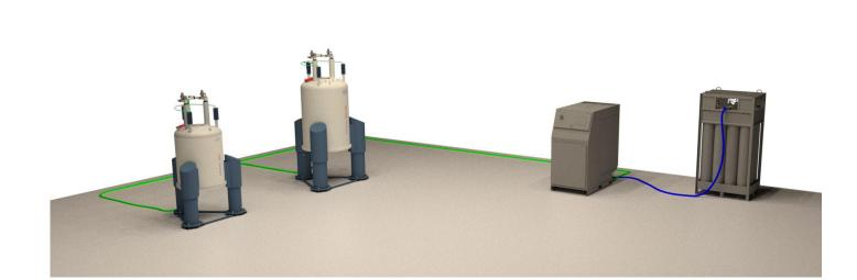
This solution is a very compact, easy-to-site helium collection unit. It collects the helium boil-off from NMR magnets and stores the gas in high-pressure cylinders. Particularly suitable for customers who have access to local or regional helium reliquefication facilities where the recovered high-pressure helium gas can be utilized.
