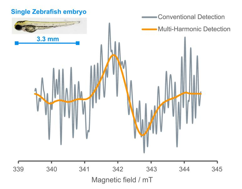
**Fig. 4** CW-EPR for in vivo study of free radicals in zebrafish embryo. Weak microwave power and aqueous samples resulting in weak signals that were improved through MHD.
