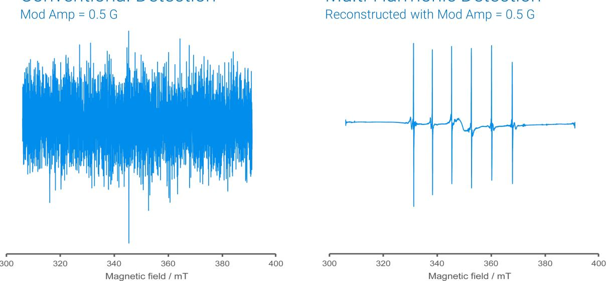
Fig. 3 Reconstruction of 1st derivative CW-EPR signal with Multi-Harmonic Detection of a Mn(II) solid sample provides large signal-to-noise enhancement.
