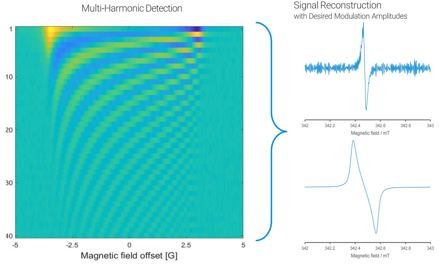
**Fig. 2** Multi-harmonic detection of a single EPR line (left). Reconstruction of 1st derivative CW-EPR signal with desired modulation amplitudes with MHD (right).
