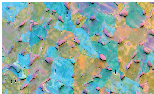
Color coded image produced by mixing the signals of the Bruker FSE detectors, showing microstructural details invisible in the grayscale image.
