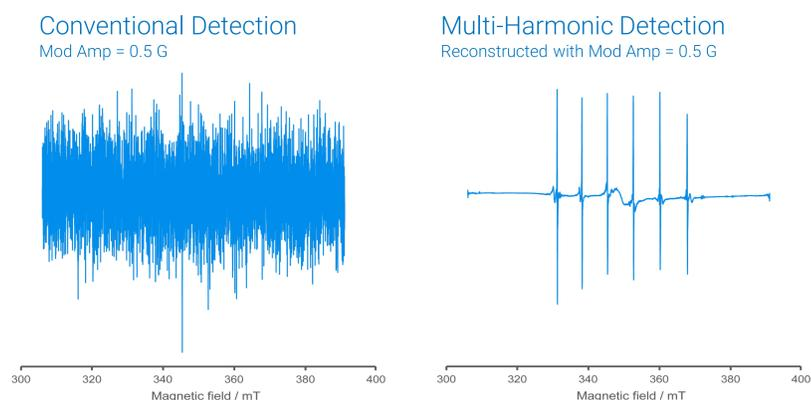
Fig. 3 Reconstruction of 1st derivative CW-EPR signal with Multi-Harmonic Detection of a Mn(II) solid sample provides large signal-to-noise enhancement.
