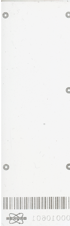
Figure 1-11 Scan created using ROI smaller than IntelliSlide, resulting in cropping of barcode and teach marks
