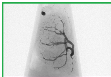
Best-Scan-Geometry means: maximum magnification and minimum scan time due to the most compact setup. Example of a plastic tube containing a mouse kidney with contrasted vasculature.
