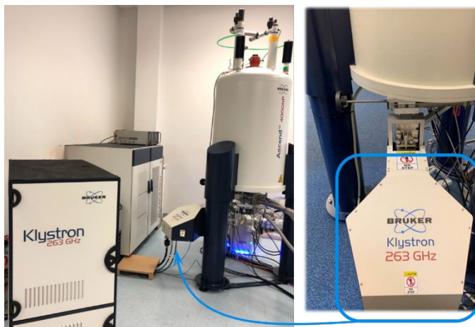
Klystron DNP installation, with control cabinet in left foreground, in front of chiller (not visible) and 2-bay solids NMR console and NMR magnet (both sold separately). The klystron mounts to a 400 MHz WB Ascend DNP magnet, highlighted at right inset.
