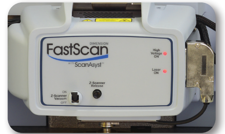
Scanner Resonant Frequency X-Y: 2.70kHz, Z: >50kHz.
