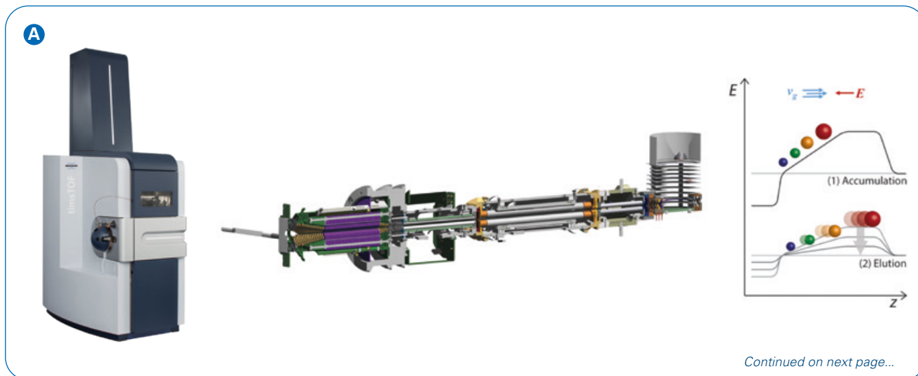
Figure 4: High confidence lipid identification workflow: A real-world example using MetaboScape 4.0. A Lipid extracts from two milk samples were analyzed by LC-MS/MS and LC-TIMS-MS/MS using a timsTOF. Shown are the instrument schematic and TIMS operation from ion accumulation to serial elution, where E represents electrical field and v_g the gas flow. B Box plot of a lipid showing different abundances in two milk lipid extracts detected in ESI positive mode. C Assignment of molecular formula based on accurate mass and true isotopic pattern using SmartFormula™ – C_{38}H_{76}NO_8P . D MS/MS query for ESI positive mode against LipidBlast library returns PC 30:0 as likely candidate. Characteristic head group fragment (184.07 m/z) substantiated assignment as glycerophosphocholine (PC). E SmartFormula3D™ algorithm: Fatty acid chains C14:0 and C16:0 could be assigned based on automatic formulae assignment for characteristic fragment ions in negative mode. F Very low deviation (0.8 %) between measured vs. predicted CCS values (279.7 vs. 277.5) provided further orthogonal confidence for the identification of the target lipid as: PC 14:0_16:0.
