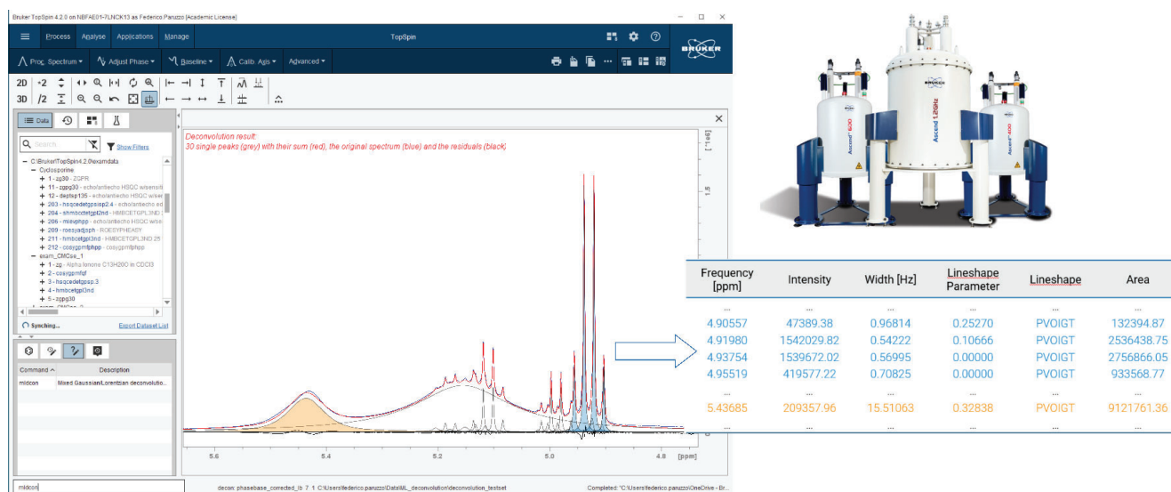
Figure 1 mldcon result on a 400 MHz ^1\text{H} spectrum. The table on the right side of the figure shows an example of the peak parameters determined by mldcon . mldcon result is visualized in the TopSpin mldcon visualization window, which displays the input spectrum (in blue), the detected peaks (in grey), their sum (reconstructed spectrum, in red), and the difference between the input and the reconstructed spectrum (residuals, in black). The algorithm stores the result as a .csv file, reporting peak position, intensity, linewidth, lineshape type and parameters, and the area of each detected peak.
