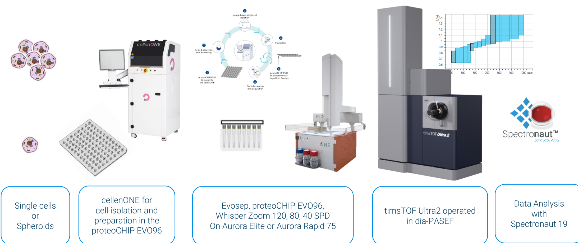
Figure 1: Single cell and Spheroid proteomics workflow with the Evosep One with Whisper Zoom 120, 80, and 40SPD using the proteoCHIP EVO96 for pipetting-free sample transfer onto Evtips Pure and pyDIAid [1] optimized dia-PASEF data acquisition on timsTOF Ultra2 with data analysis in Spectronaut 19.
