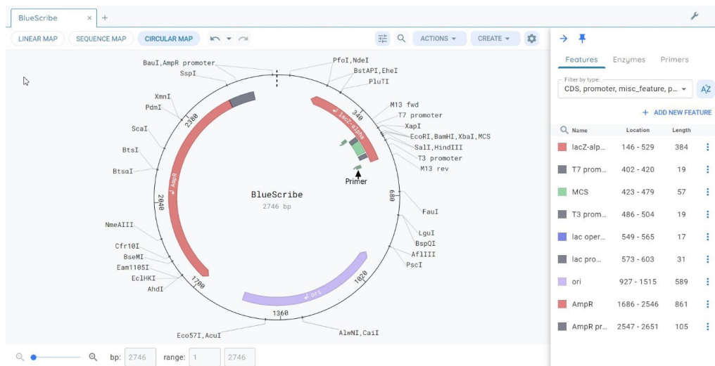
Figure 1: The Display of a circular DNA sequence with annotation features, restriction enzyme sites and primers.
