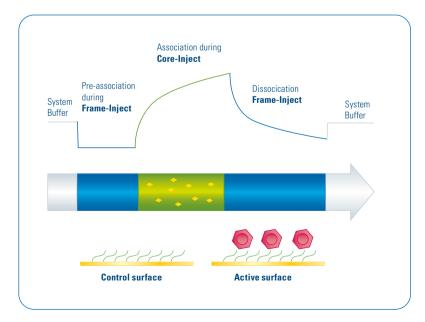
Schematic illustration of the functionality of Frame Inject. The system buffer will be replaced by the Frame solution and flow over active and control surface during pre-association phase. After the Core-Inject (Association), the dissociation is monitored while flowing the Frame solution over active and control surface. After dissociation end, Frame solution is replaced and system buffer is flowing through the microfluidic system again.
