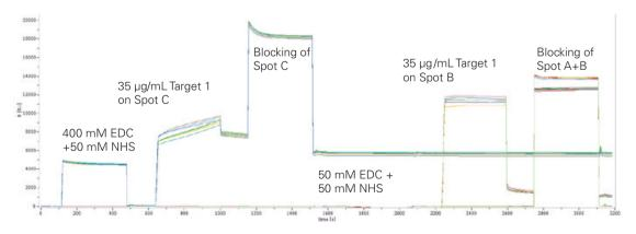
Example of surface creation using Sierra SPR-24 Pro showing high homogeneity across the eight addressed sensor spots.
